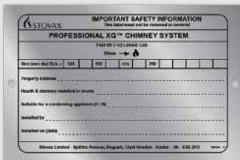
The Chimney Safety Notice Plate can be used to permanently record the flue registration and its technical specification thus complying with Building Regulations ADJ that any chimney or appliance installation must have a notice plate fixed in a visible position. Possible locations are within the fireplace or adjacent to the electricity meter, or next to the mains water stop valve.
