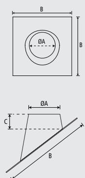
These products are used externally when the installation passes through a roof structure to provide a weatherproof seal to the surrounding weathered surface.
