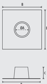
These products are used externally when the installation passes through a roof structure to provide a weatherproof seal to the surrounding weathered surface.
